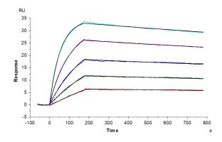
Human IL-10 R alpha, His Tag captured on CM5 Chip via Anti-His Antibody can bind Human IL-10, No Tag with an affinity constant of 0.255 nM as determined in SPR assay (Biacore T200).
